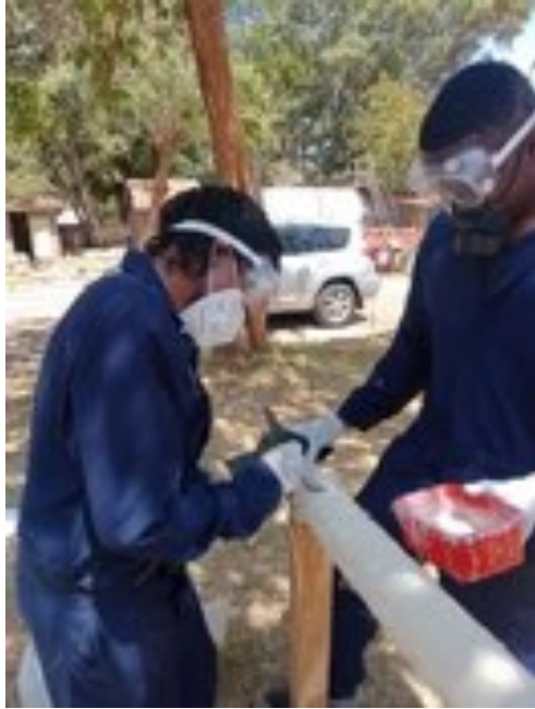
Application of resin on the fiber mat and glass
