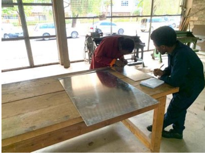
Marking out points to be drilled
